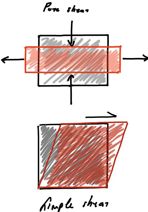
Shear modulus, also known as the **modulus of rigidity**, is a measure of a solid material's resistance to deformation when a force is applied parallel to its surface. It is defined as the ratio of shear stress (force per unit area) to shear strain (the amount of deformation).
