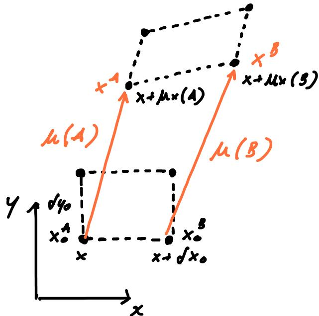
How about the **shear angles**  $\alpha$ ,  $\beta$ , and  $\gamma$ ?
