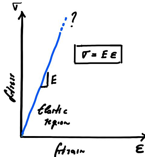
**Physically: *E* measures how much stress is needed to produce a given strain.**
