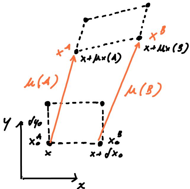
We can use these equations to define the **normal strain in  $x$ -direction**, assuming **infinitesimally small**  $\delta x_0$  and small displacements, and in analogy in  $y$ , and define:
